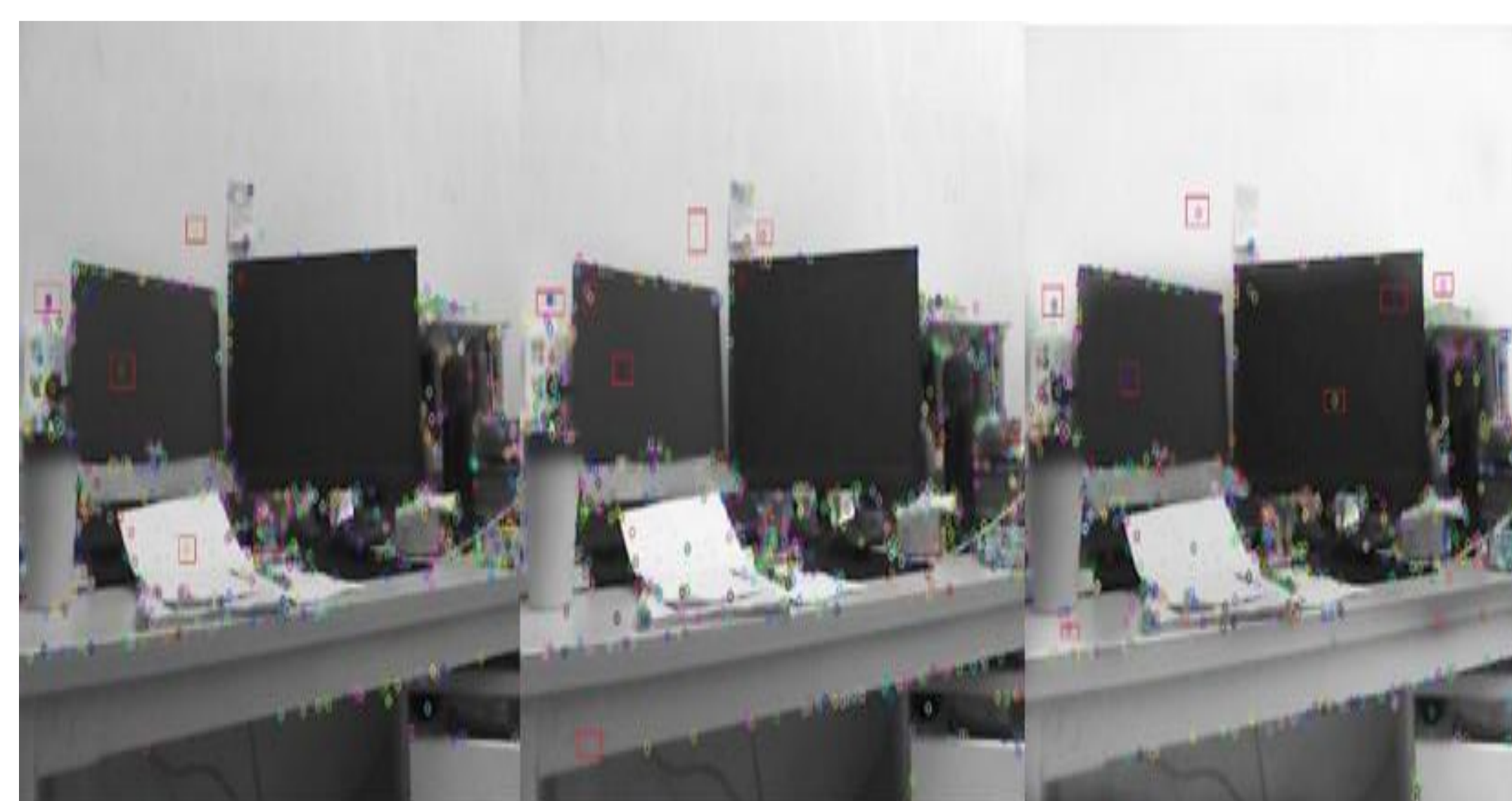
Fig.9 Running results of SIFT algorithm under different contrast in the same scene
